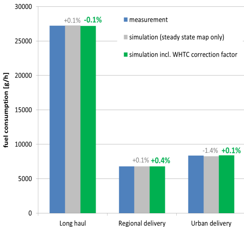
Figure 24: Comparison measured and simulated fuel consumption – engine#1
