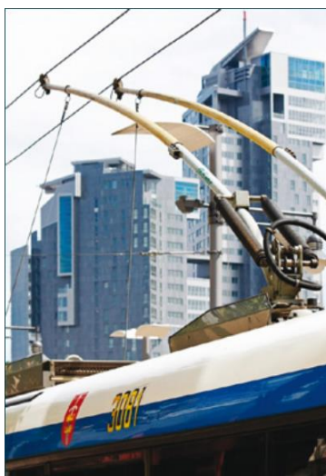
Figure 86: Trolleybus poles (photo by TROLLEY project)
