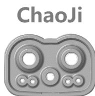
Figure 78 ChaoJi Connector interface [55]
