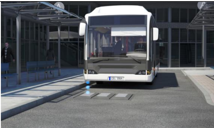
Figure 82: Floor mounted ACD Alstom solution
